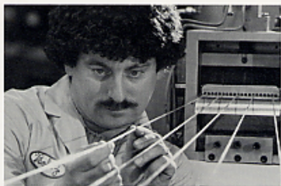
Machines producing rods for pelletizing are constantly checked to guarantee the most uniform pellets possible.
