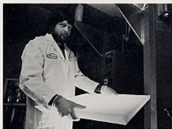
Slabs of freshly polymerized Tecoflex are removed from curing ovens to be produced into uniform sized pellets.
