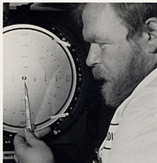
Cross-sections of Tecoflex tubing are inspected on a profile projector to ensure tight shape and dimensional accuracy.
